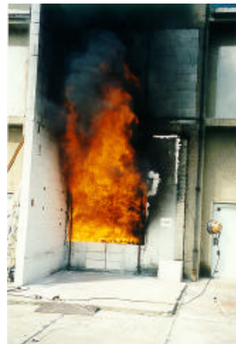
Figure 9: t = 7 min 30 s after ignition (flashover)
