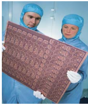
Figure 2: Printed wiring boards (PWBs) are produced by means of panels containing multiple PWBs.
